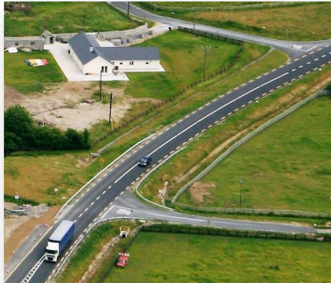
Figure 1-1: DN-GEO-03060; Simple T Junction with Right/Left Stagger
